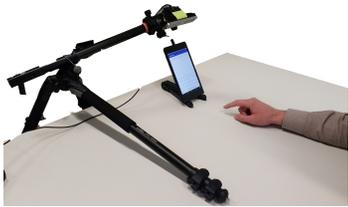
**Figure 4.** Picture of the user study setup. A tablet device provides the audiovisual feedback while a depth camera mounted on a tripod creates a virtual touch input surface.
