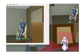
Figure 3: External people detection component (top left) uses the simulated camera images.
