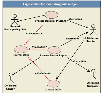
views with their associated artifacts, but also as a means to validate the software architecture for fidelity and completeness. The diagram in Figure 4b is representative of NMT's use case diagram usage and models a portion of its surveillance design.
