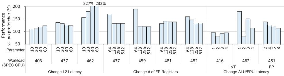
Fig. 3. Performance impact of L1 data cache prefetcher on gem5 simulator, for various architectural settings. The apparently independent parameters (i.e., register count and operation latency) affect the performance benefits. Note that we show only the sensitive workloads and parameters.
