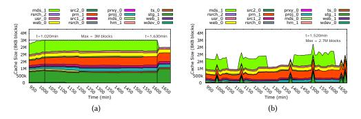
Fig. 10. Cache allocation for the VMs in infeasible state by (a) Centaur and (b) ECI-Cache.
