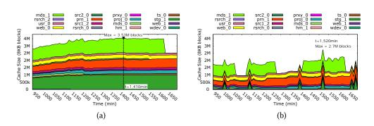
Fig. 18. Cache allocation for the VMs in feasible state by (a) Centaur and (b) ECI-Cache.
