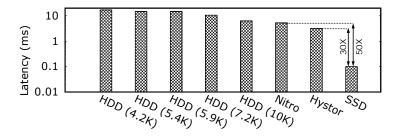
Fig. 3. HDD and SSD access latency vs. I/O caching [13, 28].
