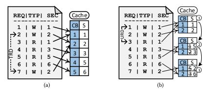
Fig. 5. Comparison of cache size allocation (a) without and (b) with considering request type (REQ: Request, TYP: Type, SEC: Sector, W: Write, R: Read, and CB: Cache Block).
