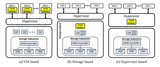
Fig. 2. I/O caching using SSDs in virtualized platforms.
