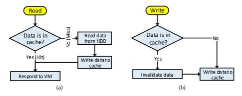
Fig. 7. Flowchart of I/O cache access for a (a) Read or (b) Write.
