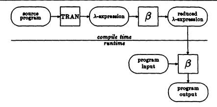
This figure shows the typical process of compilation by an automatically-generated compiler. The source program is first translated to its  $\lambda$ -expression meaning, and then  $\beta$ -reduced as far as possible. This results in a reduced  $\lambda$ -expression which is taken to be the object code for the program. The program can then be run by performing further reductions in the presence of the input file.
