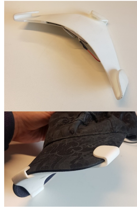
Figure 3: 3D printed head-mounted protective shell for the GNSS/IMU Sensors
