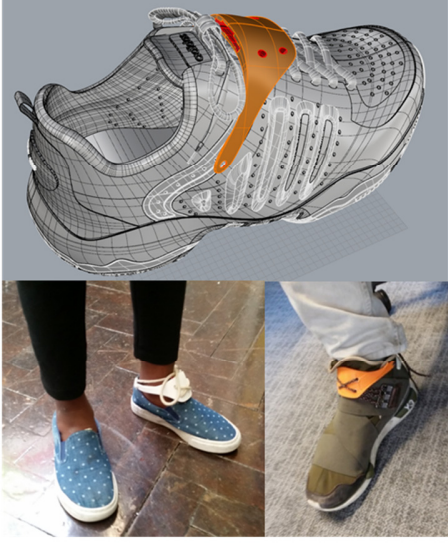
Figure 5: 3D printed show-flap protective shell for IMU
