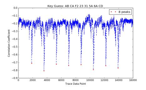
Figure 4: CPA Attack on S-Box Output
