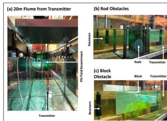
Figure 1: Flow-based molecular communication testbed with obstacles and PIV particle tracing.
