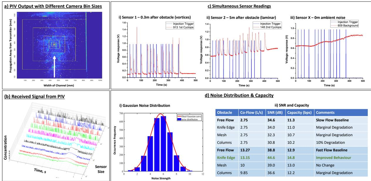
Figure 2: (a) PIV output of fluorescent dye and (b) concentration analysis as a function of time and camera capture size. (c) Received concentration at different locations, (d) noise distribution and achievable capacity with different obstacles.
