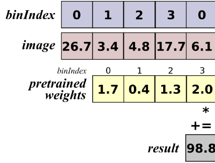
Fig. 4. Simplified weight-shared MAC example.
