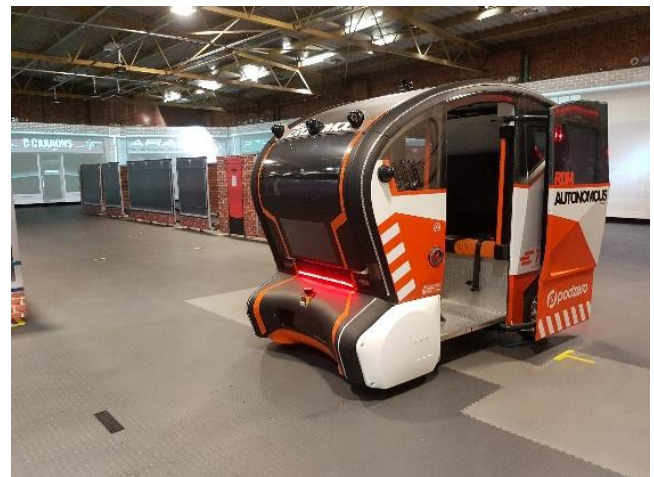
Figure 1 – The level-4 vehicle (pod), designed and manufactured by RDM Automotive, used during this study
