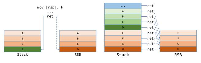
(c) Direct overwrite: A process can enforce return mispredictions by (d) Circular RSB: After returning N = 4 times, the predictor cycles replacing return addresses stored on the stack. over and will repeat the same prediction sequence of return addresses.
