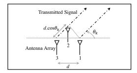
Figure 3. Uniform linear array consisting of 3 antennas: For AoD of  $\theta_k$ , the target's signal travels an additional distance of  $d\cos(\theta_k)$  from the second antenna in the array compared to the signal from the first antenna. This results in an additional phase of  $-2\pi d\cos(\theta_k)/\lambda$  for the signal received from the second antenna compared to that from the first antenna.
