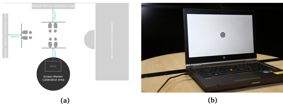
Figure 5.15: Screen Marker Calibration Area, position illustrated in the left, and an image of the real setup in the right. Calibration is performed on a screen.
