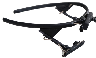
Figure 4.1: A binocular Pupil Labs eye tracker, with two infrared cameras, which are capturing each eye, and a wide-range world camera, that is recording the egocentric view.
