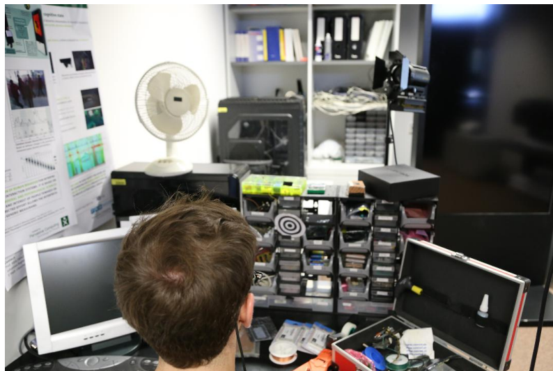
Figure 5.20: Accuracy evaluation using visual markers placed within a fictional working place.
