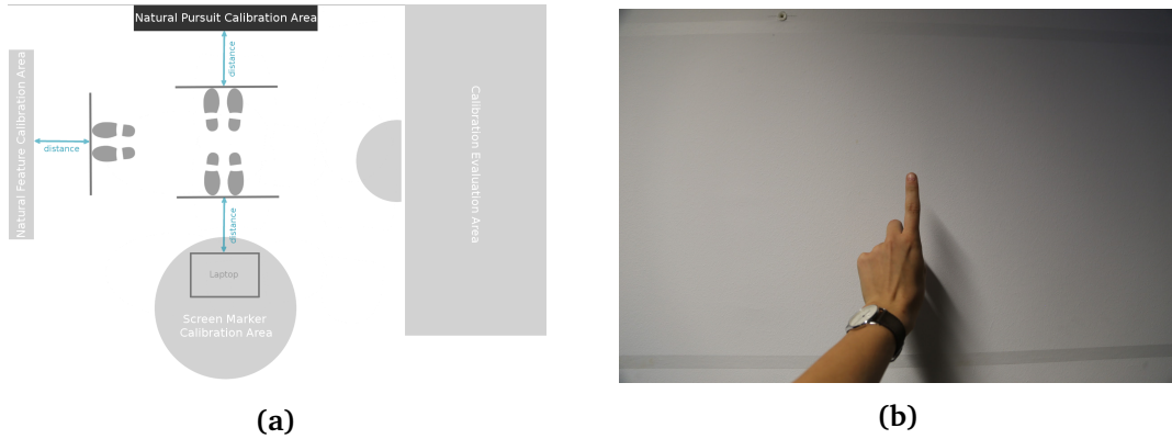
Figure 5.18: Natural Pursuit Calibration Area, position illustrated in the left and an image of the real setup in the right. Only the person's finger is used for calibration.
