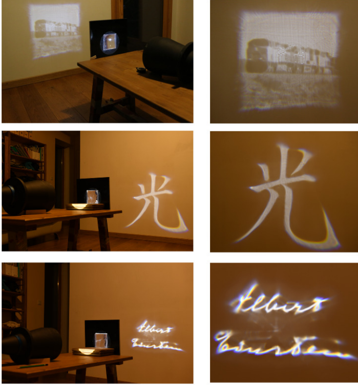
Figure 16: Fabricated lenses for a collimated light source. From left to right: experimental setup, zoom on the target screen. From top to bottom: TRAIN, HIKARI, EINSTEIN'S SIGNATURE targets. Images are focused on a screen at 2 meters for the first two rows and 1 meter for the last one.
