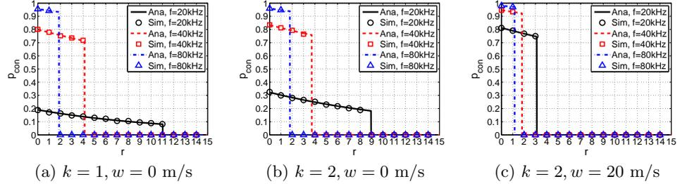
Figure 3: Probability of connection  $p_{con}$  versus distance  $r$  with different spreading factor  $k$  and wind speed  $w$ . System parameters are set by  $P_p = 110$  dB,  $P_s = 100$  dB,  $\lambda_p = 0.003$ ,  $s = 1$ ,  $\delta_s = 20$  dB and  $\delta_d = 20$  dB
