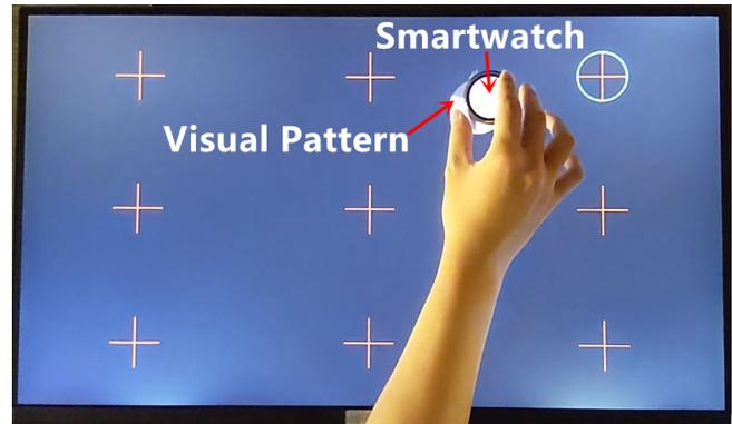
Figure 1. User grabbing and moving a smartwatch on top of a non-touchscreen. The location of the smartwatch is continuously tracked with high frame rate and minimal delay using IMU. If the estimated location is different from the ground truth, the visual pattern beneath the watch will expand or shrink. The changes will be tracked by PPG sensor, and the pattern shift accordingly to minimize error caused by drift.
