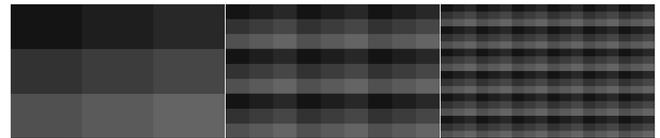
Figure 3. Flashing the whole screen with grid to search and localize the initial location of the smartwatch iteratively. From left to right, this figure depicts three iterations.
