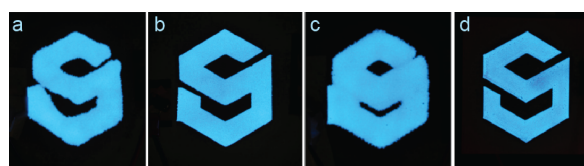
Figure 5. Test 2: four EL cells sprayed onto flat substrates using techniques to define cell shapes on the base electrode: a) hand masking; b) contact masking; c) shadow masking; d) 3D printer-shaped cells.
