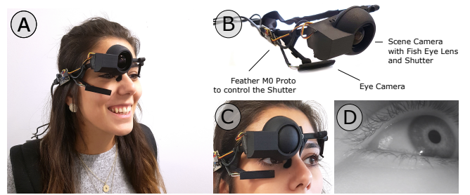
Figure 2: PrivacEye prototype with labelled components (B) and worn by a user with a USB-connected laptop in a backpack (A). Detection of privacy-sensitive situations using computer vision closes the camera shutter (C), which is reopened based on a change in the privacy detected level in a user’s eye movements (D).
