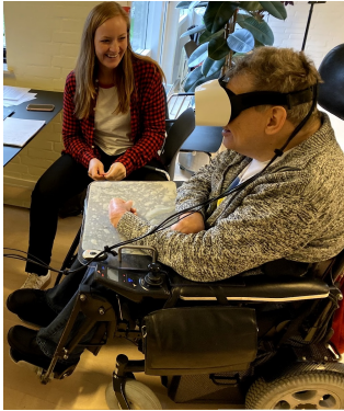
Figure 3: A participant wearing an HMD with a built-in eye tracker.
