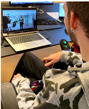
Figure 4: A participant using the Double robot in front of a screen and the Tobii eye trackers. In this case the experimenter was standing behind the user and emulating his gaze movements by use of a joystick, applying a Wizard of Oz technique.
