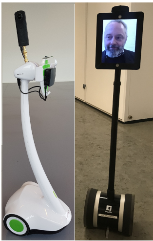
Figure 2: The two robots applied in the field study: a) A Padbot robot (left) that we attached with a 360 degree camera (but without a monitor showing the users face); b) A Double robot (right) with a live face video.
