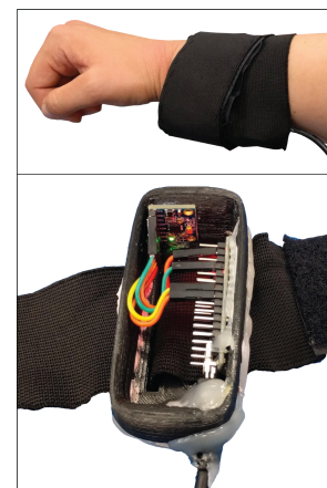
Figure 2: Top: the prototype attached to the inside of a hand. Bottom: inside of the prototype.
