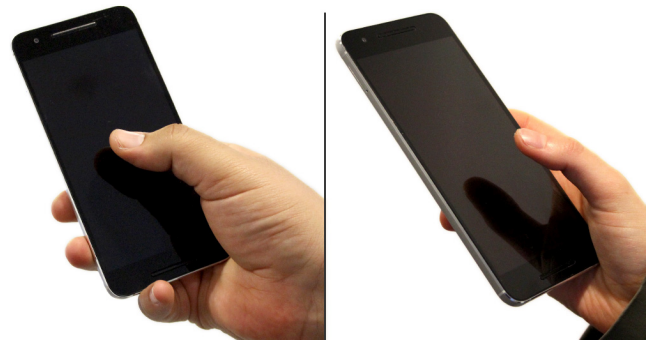
Figure 1: We investigate how touch error varies between users with different hand sizes. Seen here are a user with a large hand (left) and a smaller hand (right) holding the same phone. We find that thumb length in particular correlates significantly with touch error.
