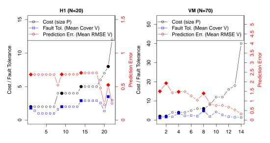
Fig. 4. Examples of Pareto-fronts (highlighted points) to minimize cost and prediction error and maximize fault-tolerance.
