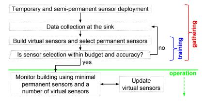
Fig. 1. The three phases of the BuildSense framework.
