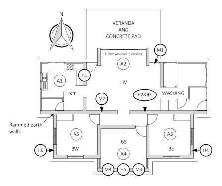
Fig. 5. House plan and sensor placements for both the monolithic and insulated houses. See the text for an explanation of the sensor labels.
