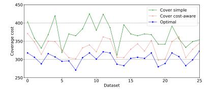
Fig. 7. Coverage cost of the permanent sensor deployment based on the three sensor selection algorithms, where coverage cost is equivalent to the total purchasing cost of the deployed nodes in *AUD*.
