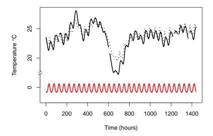
Fig. 2. Sensor readings from a bedroom (dotted) and embedded in a wall (black) and their average difference by the hour of day (red).
