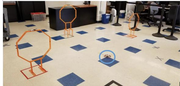
Figure 7. Lab configuration for an experiment with three hoops set up at different heights as obstacles. The miniature Crazyflie UAV (circled in blue) can fit through these hoops with approximately a body length on either side.
