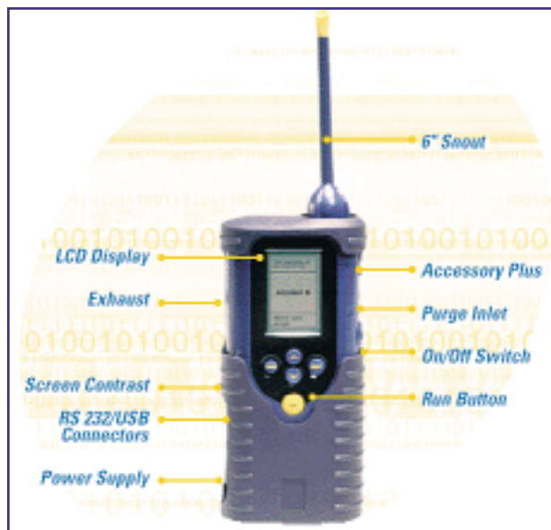
The Cyranose 320, from Cyrano Sciences, can recognize smells.
