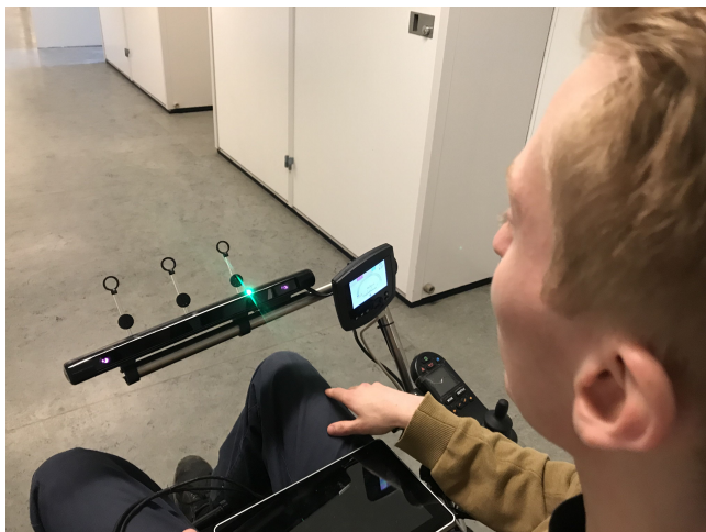
Figure 12: Driving with the "GazeDriver" in a real world felt much like driving it in the simulator. The green light indicate that the user is making a right turn because he looks through the right circle
