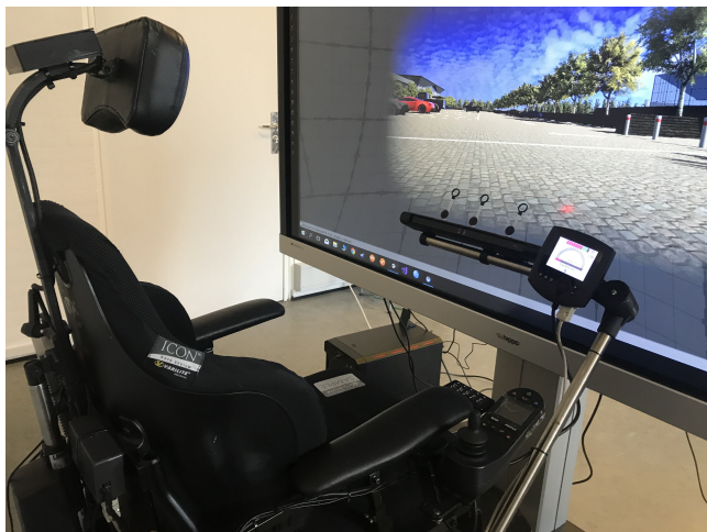
Figure 11: Testing the "GazeDriver" in a wheelchair simulator. The wheel-turns are transformed to movements in a VR game environment shown on the big monitor in front of the user. The user looks through the 3 circles above the tracker to steer left, straight, or right.
