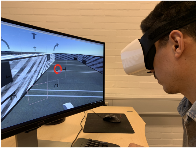
Figure 1: Experiment setup with the view from the head-mounted gaze-tracking display shown on the monitor. The participant turns to the right by dwelling at an overlay key (indicated by a red progress circle)
