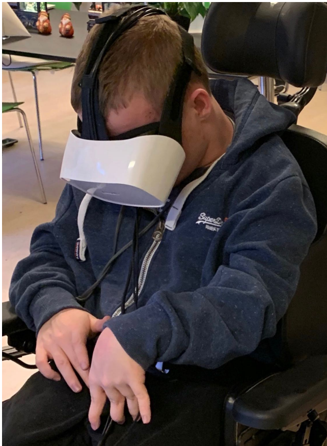
Figure 9: Testing gaze controlled navigation in a long-term care facility. Participants complained that looking to the floor-plan felt uncomfortable and made it difficult to see the surroundings.
