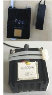
(b) Peltiers and vibrotactile Haptuator
