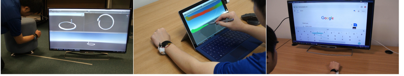
Figure 7: Left: 3D object measurement tool. Middle: Bimanual interaction for controlling stylus properties. Right: Anywhere cursor control for inputting text using gesture keyboard technique.
