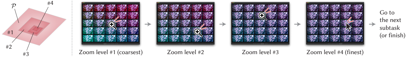
Fig. 3. Zooming procedure in the zoomable grid interface. The user clicks the best option displayed in the grid, and then the interface goes to the next finer zoom level. After a certain number of clicks (four in this example), this plane-search subtask ends. If the user wants to continue exploration, our method constructs a new search plane and then asks the user to start another zooming procedure.
