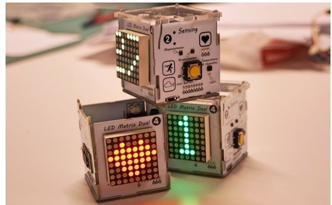
Figure 2: The Magic Cubes toolkit comprises hand-sized cubes with embedded sensors and collocated numeric or symbolic visualizations.
