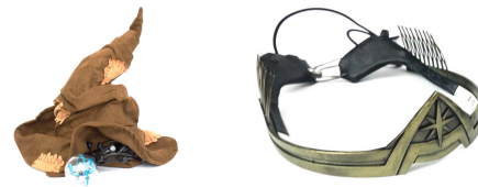
Figure 3: Examples of assembled “Magic Hat” system. Left: The Sorting Hat from Harry Potter with Emotiv Epoc headset inside as well as a Sphero robotic ball next to it. Right: a tiara from Wonder Woman with a Muse headband inside.
