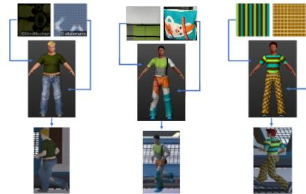
**Figure 5: Examples of generated clothes. From top to bottom: UV texture maps, 3D characters wearing the new clothing after UV mapping, images rendered in a Unity scene. From left to right: 3D characters generated using the clothing models with the original UV texture map, a UV map with a web image, and a UV map with a random color and texture pattern.**
