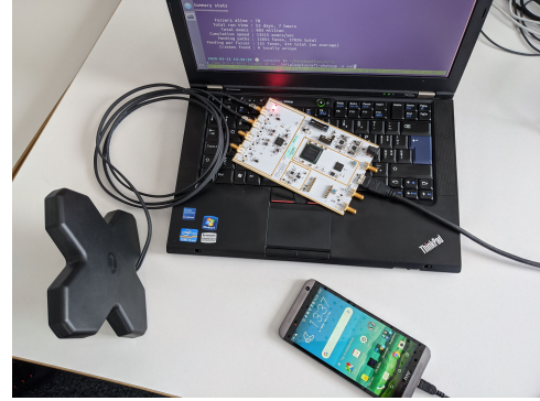
Figure 6: Base station setup with our test phone HTC One E9.
