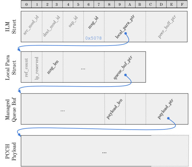
Figure 4: Structure of MTK ILM, encapsulating a PCCH Message including pointers needed for correct input placement.
