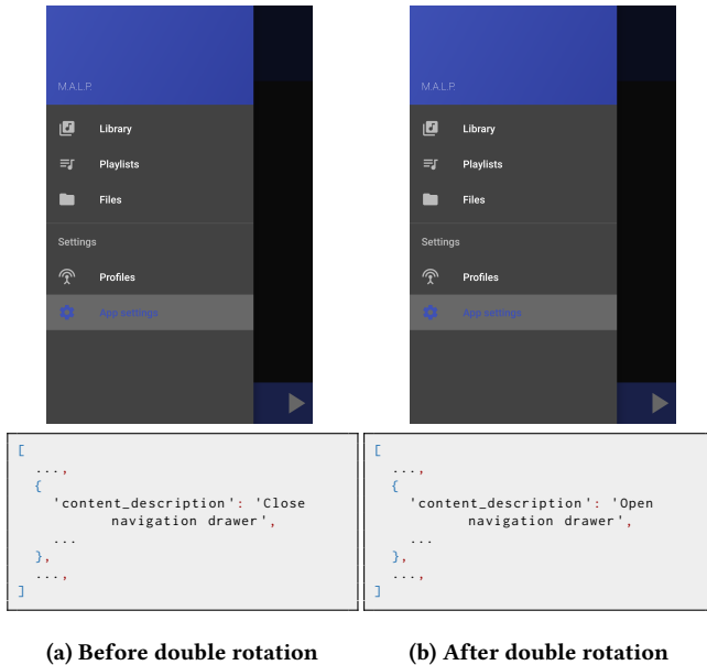
Figure 3: A data loss failure detected by the property-based oracle only in MALP 3d31062.
