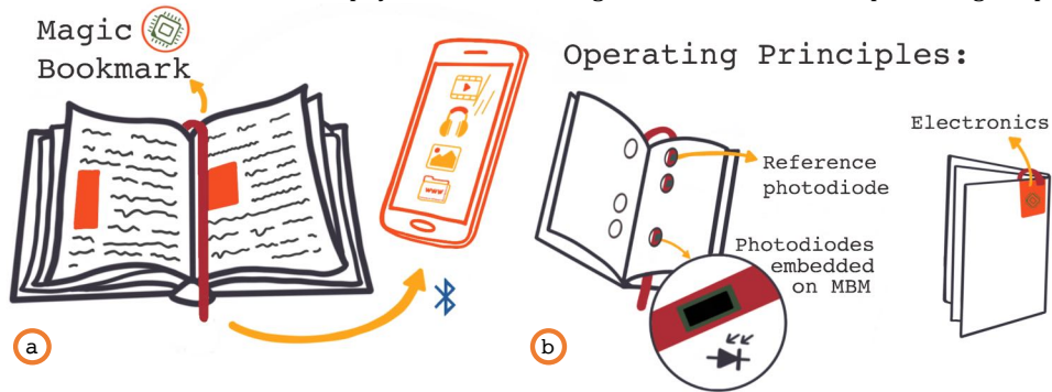
Figure 4: The Magic Bookmark concept (part a) and the main operating principles (part b).
