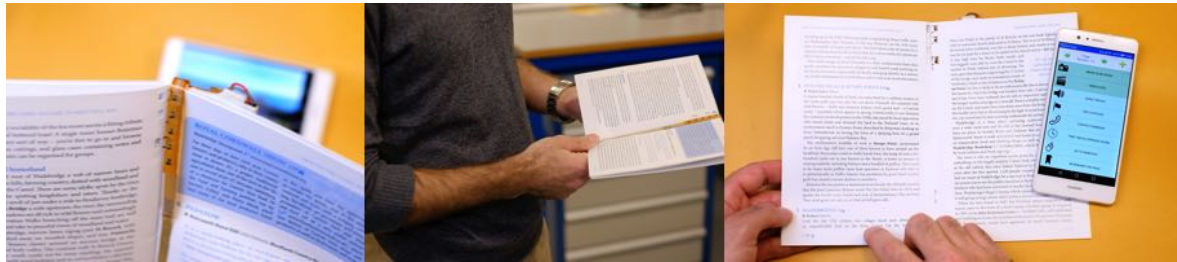
Figure 5: The second demonstrator, the Magic BookMark, in use. This prototype is utilizing the first method for open page detection. The bookmark is placed behind the active page and the content consumption is handled by the Next Generation Paper ecosystem.
