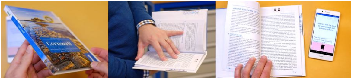
Figure 2: The first demonstrator, the Light Tags, is used in the 3G a-book device for open page detection. Pressing the buttons on the side of the book triggers the corresponding digital media on the phone connected to the hybrid device.
