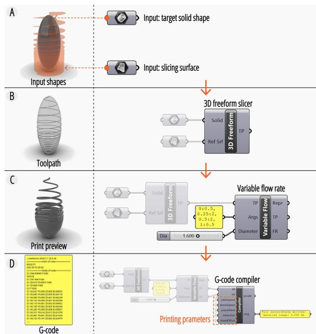
**Figure 10: Chocolate jelly art toolpath design walkthrough - (A) modeling input solid and slicing surface as inputs, (B) creating a freeform toolpath using the 3D freeform slicer, (C) assigning the toolpath with a variable flow rate profile, and (D) generating a .gcode file by specifying the printing parameters.**
