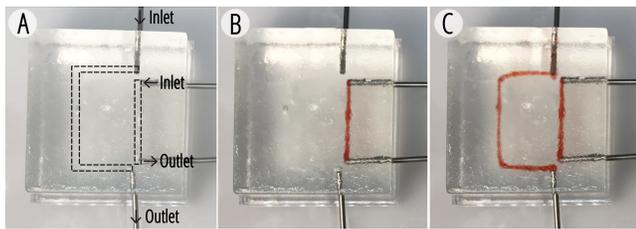
**Figure 15: Jelly display - (A) design schematics, and (B) perfusing one segment to show ‘1’ and (C) both segments to show ‘0’.**
