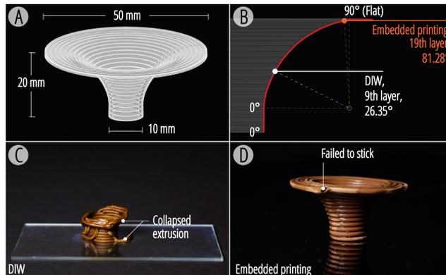
**Figure 6: Freeform printing test - (A) the model used for this experiment has (B) an increasing overhang along the z-axis. (C) The model printed with DIW and (D) embedded printing in a Carbopol support bath.**
