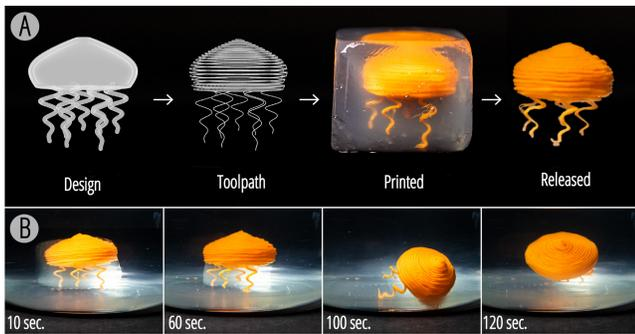
**Figure 13: A jellyfish made of the alginate-carrot ink - (A) target shape, printing toolpath, and printed and released jellyfish. (B) The release process showing the gelatin dissolving away in a water bath (60°C) and the jellyfish becoming adrift.**
