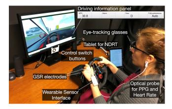
Figure 2: User study setup. This custom driving simulator consists of a 30-inch monitor, a Logitech G29 steering wheel, and 10.5-inch Apple iPad Air on which the non-driving tasks are displayed. For switching between the automated and manual control of the vehicle, the participant needs to press the two blue buttons on the steering wheel simultaneously. The participant wears a pair of eye-tracking glasses, and a wearable device with GSR and PPG sensors for the biometrics acquisition.
