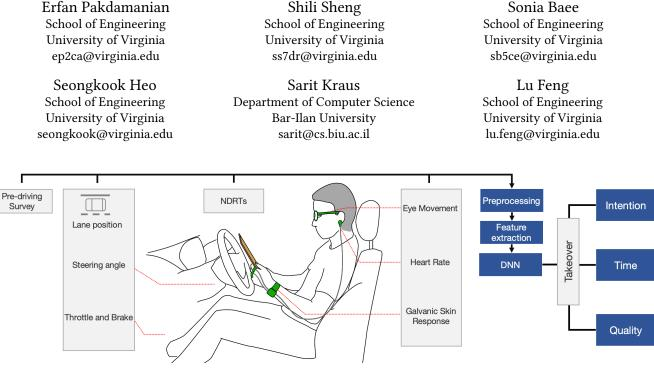
Figure 1: DeepTake uses data from multiple sources (pre-driving survey, vehicle data, non-driving related tasks (NDRTs) information, and driver biometrics) and feeds the preprocessed extracted features into deep neural network models for the prediction of takeover intention, time and quality.
