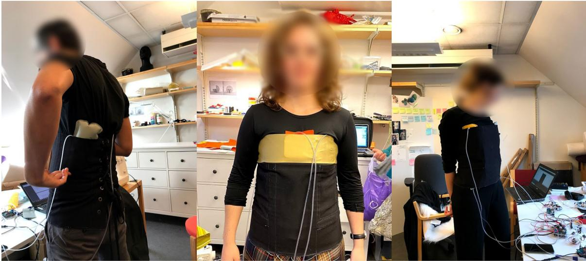
**Figure 7: Wearing the Breathing Shell and testing the somatic impact of non-habitual breathing, through the shape-change sensor-actuator pillows. The tubes lead to the areas where the pillows are placed.**
