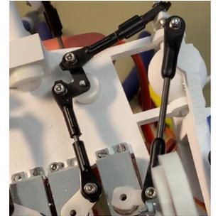
*Computing global costs.* As mentioned, global costs can have several use cases. In this work we use it to prevent designs that lead to self-collisions between the mechanical elements used to transmit forces from motors to the armature. We identify worst-case collision configurations using an approach inspired by the concept of adversarial attacks. More precisely, we actively drive the mechanism towards configurations where the internal components get as close
