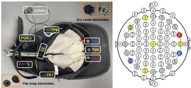
**Figure 2: Soft EEG cap and electrode placement.**
