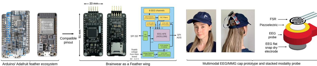
Figure 1: Left: Brainwear is compatible with the Adafruit Feather footprint. Right: aesthetical wearable for HAR and multi-modal probe.
