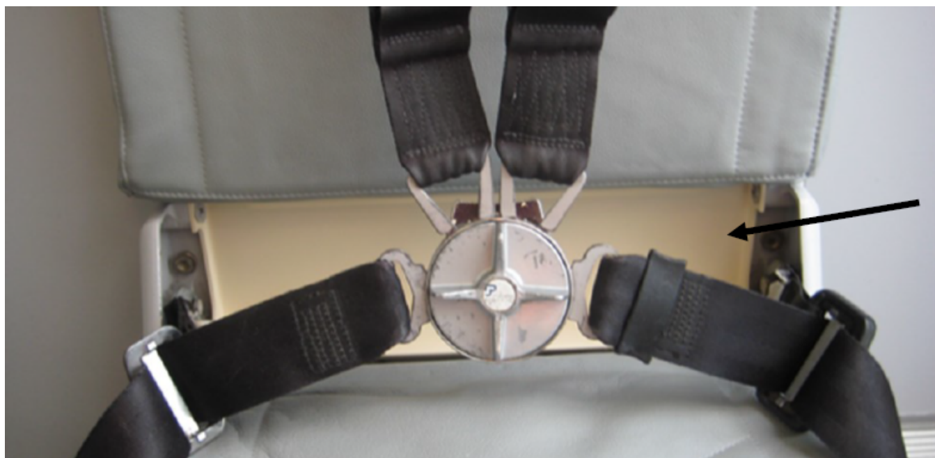
Figure 1: Installed belt mold spare part for the Airbus A300/A310 additively manufactured on demand.
