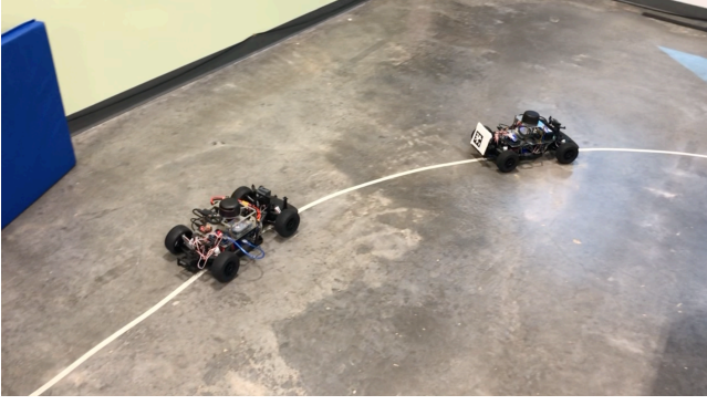
Figure 6: Both vehicles follow the line marked with the vehicle behind maintaining a constant distance.
