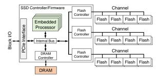
Figure 2: Internal architecture of flash-based SSDs.
