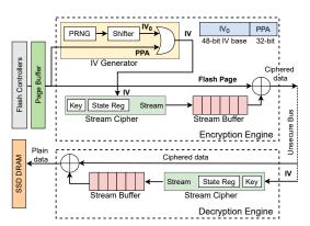
Figure 10: Stream cipher engine design in IceClave.
