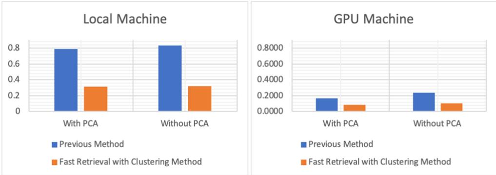
Fig. 25. Comparison of tested average image retrieval time on DBCaltech between proposed Fast Retrieval method and previous method. The standard deviation of the image retrieval time is about 0.01 s.
