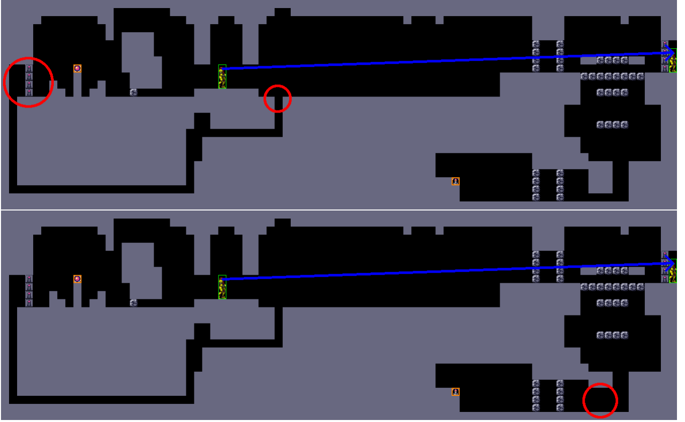
Figure 4: Two modified abstract levels (a) and (b) based on the real level shown in Figure 3. The path on the left (entrances circled) has been added to illustrate how the system detects softlocks. In each level, the blue arrow points from the start state to the goal state. Design (b) is identical to (a) except where circled. Design (a) satisfies AG(EF(goal)) , while design (b) does not. Figure 5 shows why (b) fails this verification. The two item upgrades (missiles and morph ball) are highlighted in orange.
