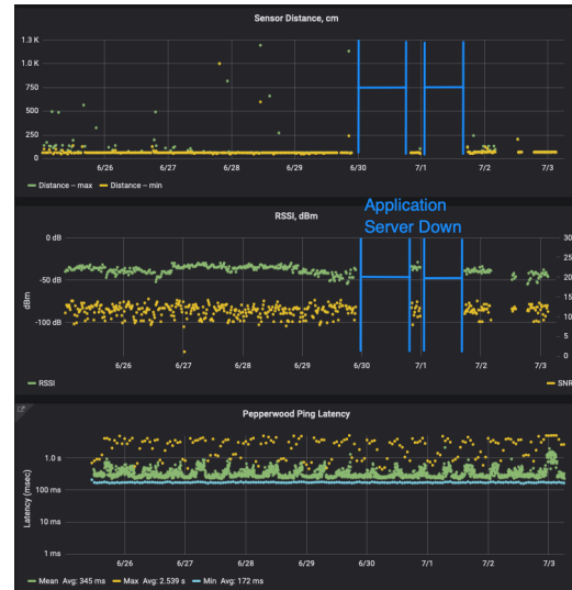
Figure 4: Grafana dashboard with data traces for distance (analogous to water level), RSSI, and gateway ping latency. Some periods lack sensor data due to an application server issue.
