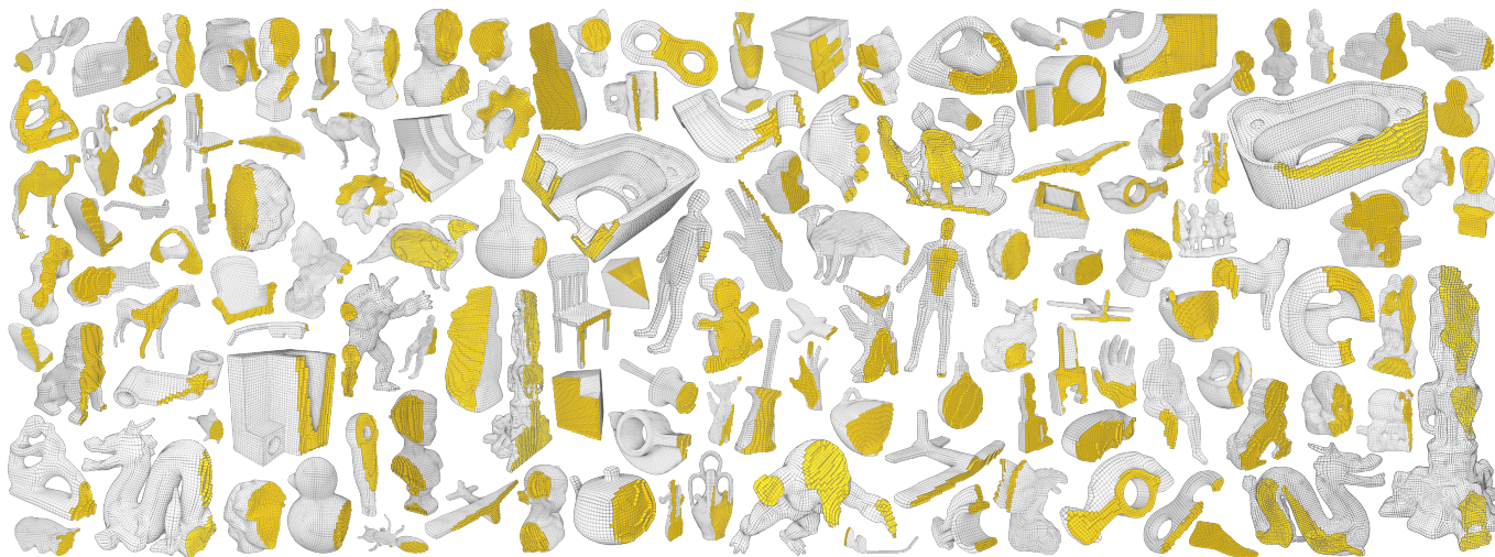
Fig. 1. A sampling of hexahedral meshes produced by our method. Our user-in-the-loop interactive pipeline facilitates the creation of high-quality hex meshes, giving the user the option to control the final result at any desired level of granularity.
