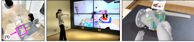
(a) (left) Third-person view of the VR. (center) The remote expert demonstrates ball valve locking. The display wall presents the scene being viewed by the remote expert. (right) Screen viewed by the local worker.
