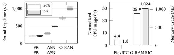
**(a) Round-trip times for two hops. (b) CPU and memory usage.****Figure 9: Comparison of O-RAN RIC and (dockerized) FlexRIC.**
