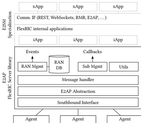
**Figure 5:** The FlexRIC server library provides communication means and an E2AP abstraction. Specialized controllers are implemented through internal applications (iApps). They provide services to external applications (xApps) through custom, controller-specific northbound interfaces.
