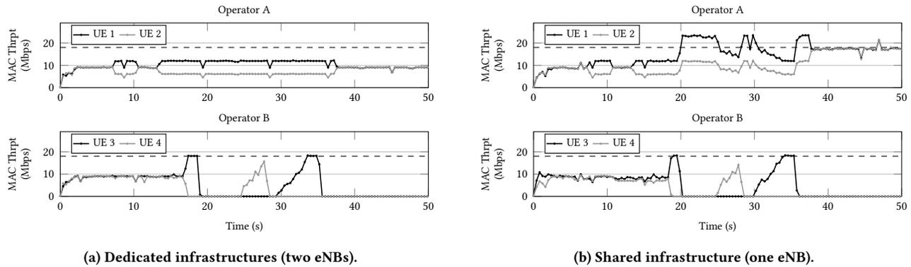
**Figure 15: Comparison of dedicated and shared infrastructure of two operators with (in total) four UEs. The controllers can freely reconfigure slices. In the sharing case (b), isolation and sharing properties are preserved.**
