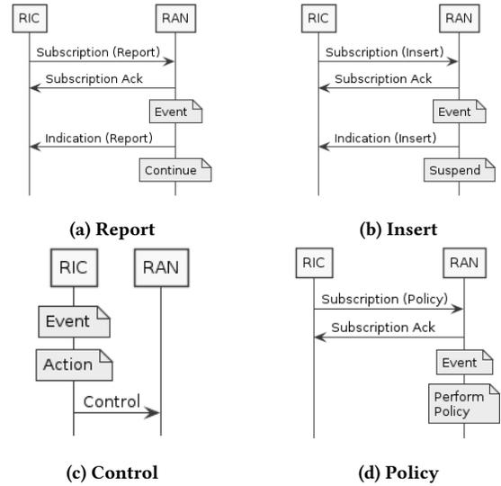
**Figure 17: The four basic “services” that are specified in E2SMs to define the interaction between an xApp and a RAN function.**
