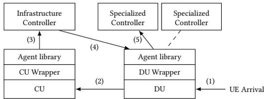
**Figure 4:** For disaggregated base stations, a controller needs to configure the UE-to-controller association in all agents (step 4) to ensure that a connecting UE (step 1) is exposed to the specialized controller (step 5).
