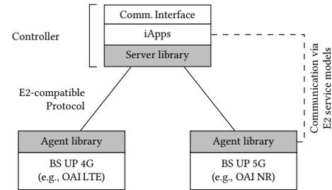
**Figure 1: The FlexRIC SDK consists of an agent and a server library. The agent library provides integration of a base station to a controller, which is specialized to a particular use case using iApps.**
