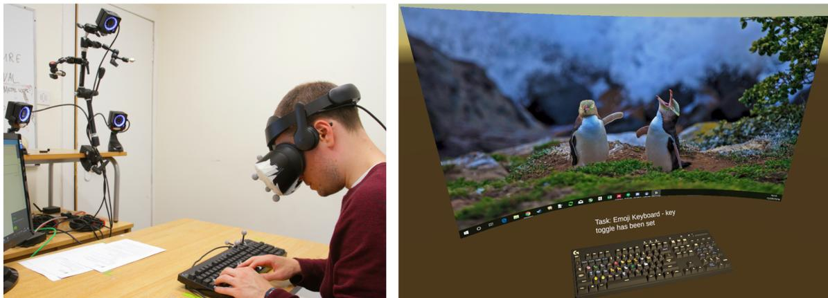
Fig. 2. Left: Experimental setup, with 3 Optitrack 13W cameras tracking markers attached to the participant's fingers, as well as rigidbodies attached to the keyboard/VR headset. Right: View in VR, with a virtual display showing the Windows desktop and an aligned virtual representation of the physical keyboard.
