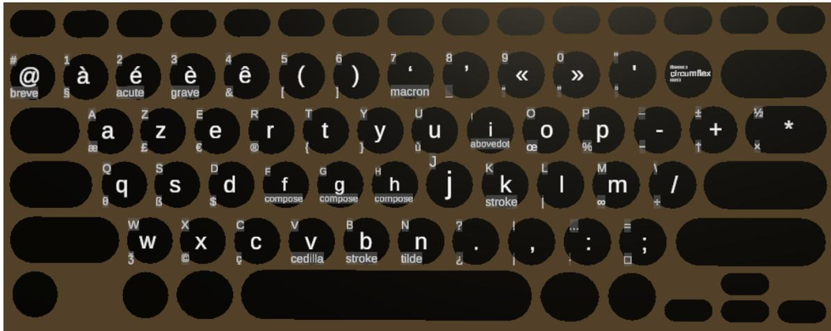
Fig. 10. Example of the new AZERTY [25–27], imported as JSON generated by KLFC using the XKB definition [29], with alternate/shift keys also visualized.
