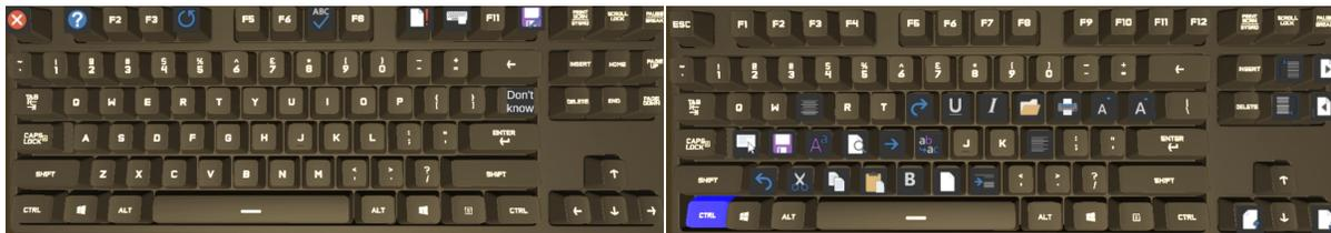
Fig. 5. VR Keyboard layouts for the **Icon** condition with (top) non-modified F-key shortcuts being visualised and (bottom) CTRL-modified shortcuts being visualised when the CTRL key was pressed.
